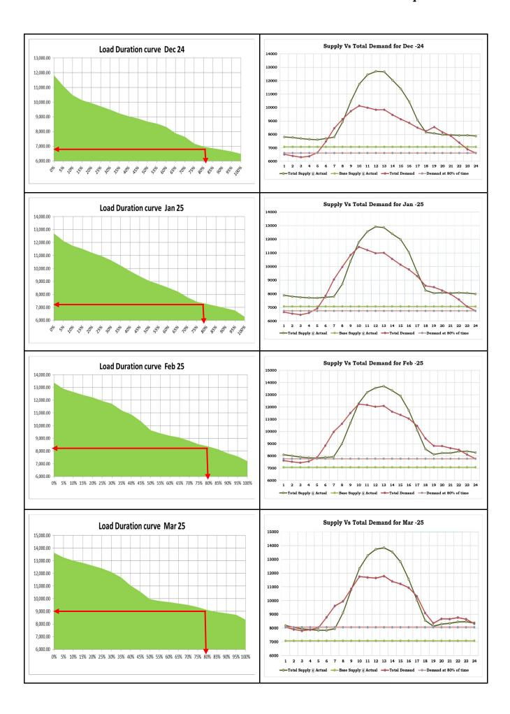
Based on the load duration curves and base supply availability, the shortage/surplus of base generation capacity in MW for a whole year and each month at 100 per cent time of base load and 80 per cent of the time of base load are computed as shown in the Annexure-13 and the conclusion of which for a whole year and each month is shown in the table below.
